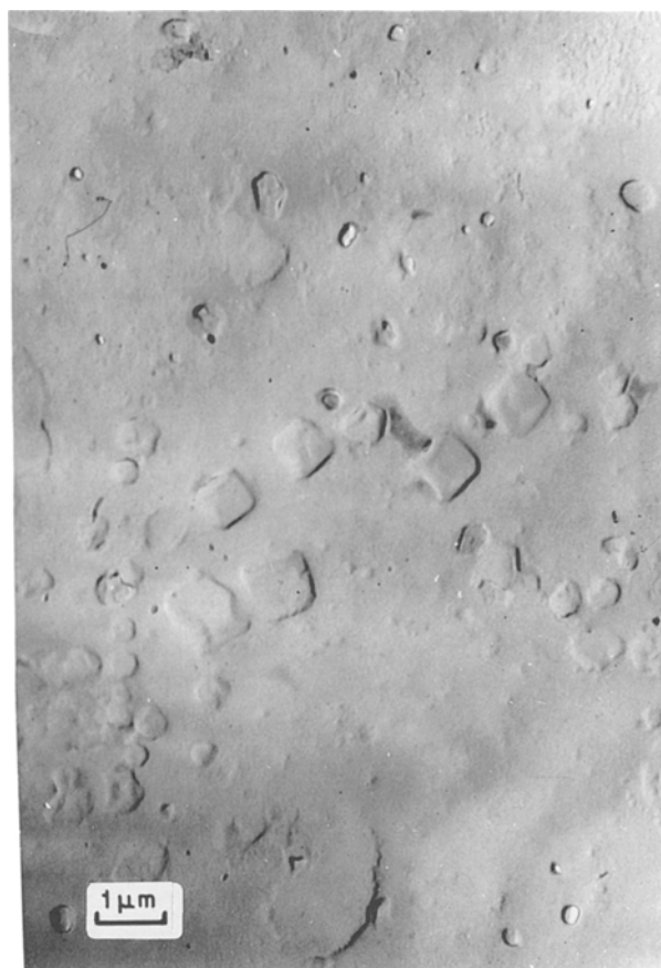
Figure 9 Transmission electron micrograph of fritted \text{CaF}_2 (B) using a Pt/C replica from the freshly broken sample. \text{CaF}_2 crystallites are visible.
